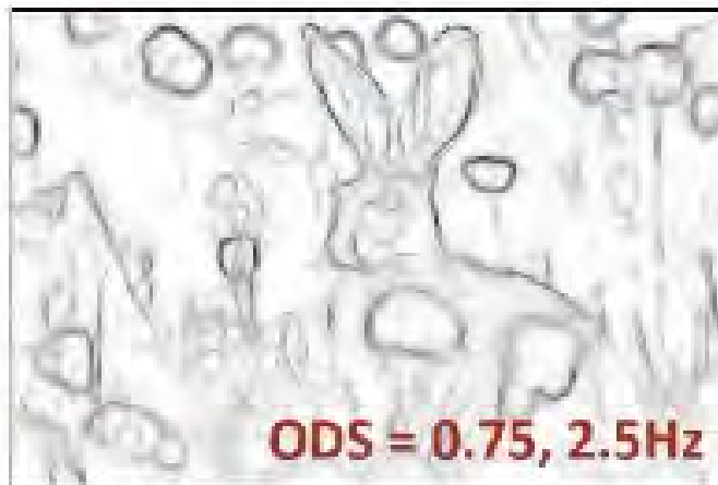
Fig. 1. Edge detection results using three versions of our Structured Edge (SE) detector demonstrating tradeoffs in accuracy vs. runtime. We obtain realtime performance while simultaneously achieving state-of-the-art results. ODS numbers were computed on BSDS [1] on which the popular gPb detector [1] achieves a score of .73. The variants shown include SE, SE+SH, and SE+MS+SH, see §4 for details.
