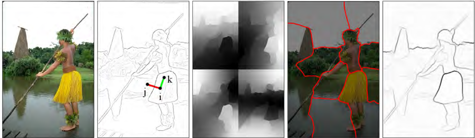
Fig. 7. Spectral Pb. Left: Image. Middle Left: The thinned non-max suppressed multiscale Pb signal defines a sparse affinity matrix connecting pixels within a fixed radius. Pixels i and j have a low affinity as a strong boundary separates them, whereas i and k have high affinity. Middle: First four generalized eigenvectors resulting from spectral clustering. Middle Right: Partitioning the image by running K-means clustering on the eigenvectors erroneously breaks smooth regions. Right: Instead, we compute gradients of the eigenvectors, transforming them back into a contour signal.
